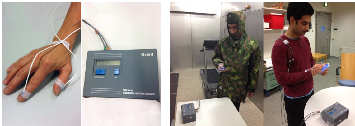
Fig. 2. Left: Grant Squirrel meter/logger (series 1000) and a participant's hand with thermal sensors attached. Right: Participant in the cold chamber and in the warm room.
